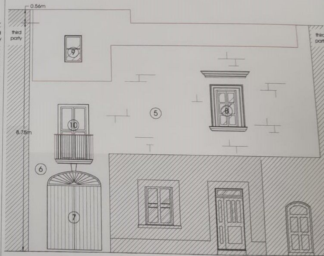
B Proposed Front Elevation Ref 02B Scale 1:50
