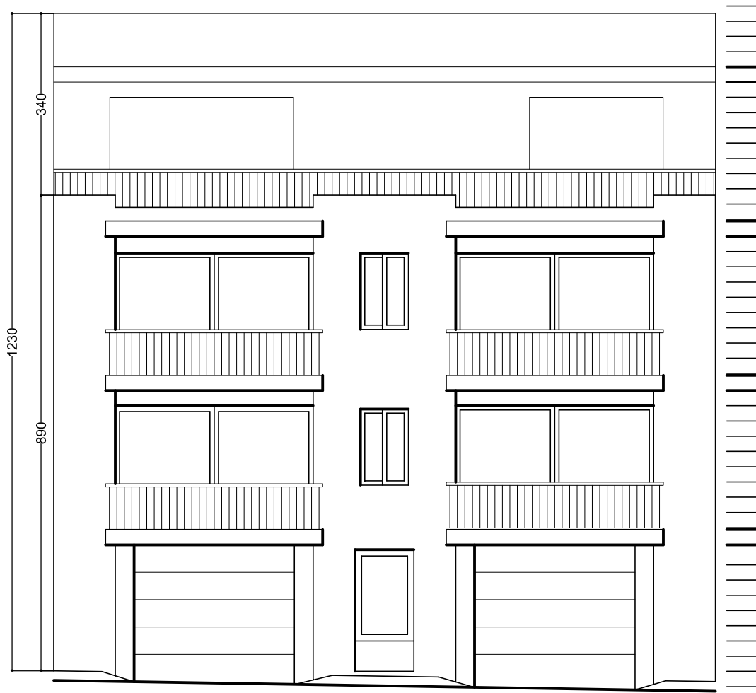
○ Front Elevation 1:100 As Proposed Unpainted Franka Stone Facade White aluminum apertures and railings
